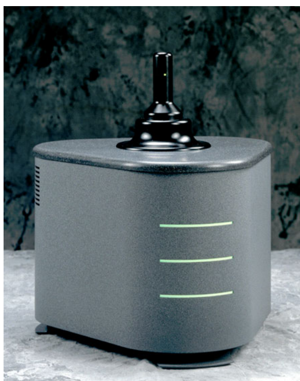
B – CSC Nano ITC III 5300 modelio kalorimetras
